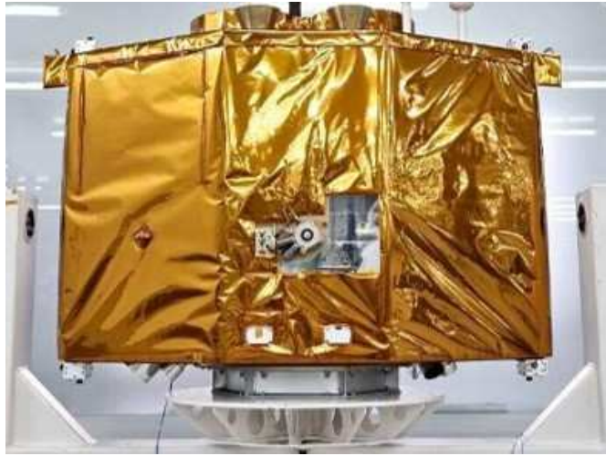
FIGURE 9. EOS SAT-1 spacecraft with SPS-25 propulsion system.
