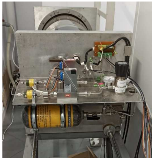
FIGURE 2. Laboratory feeding system for the laboratory testing.
