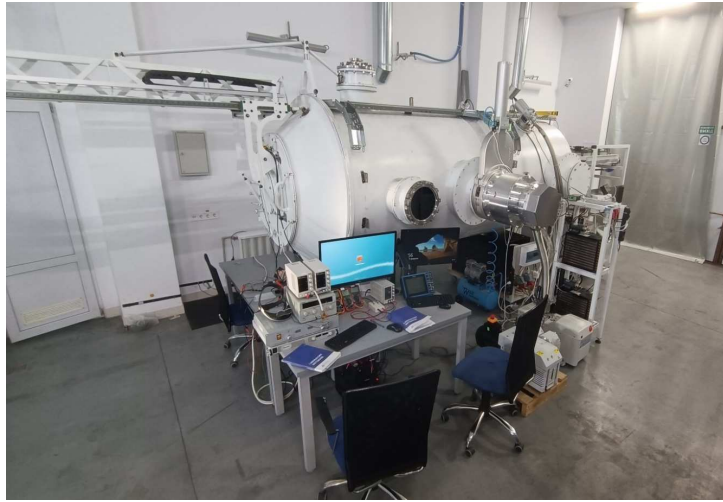
FIGURE 1. Vacuum chamber for the laboratory testing.
