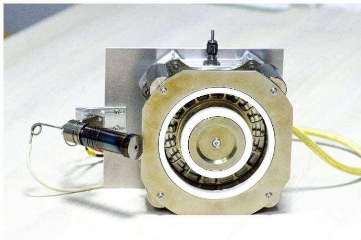
FIGURE 16. General view of the ST-100 Hall thruster.
